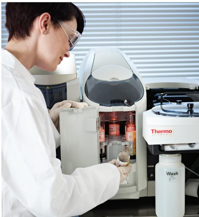
Figure 1. Thermo Scientific iCE 3000 Series AA Instrument.
