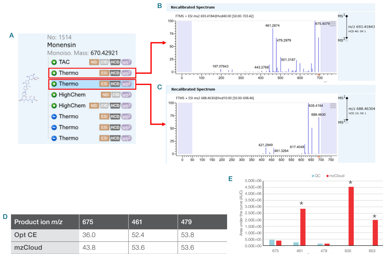
Figure 7. The mzCloud database entry for monensin and the different instances in +ESI and -ESI (A). The representative HCD product ion spectra are from precursors formed by two instances resulting from B) a sodium and C) an ammonium adduct were evaluated using the import function on the TSQ Plus mass spectrometer in the same method. The resulting comparison of CE values used for the sodium adduct are shown in D) and E) the comparative AUC responses measured for each SRM transition. The transitions with asterisks were acquired using the monensin precursor formed by an ammonium adduct.
