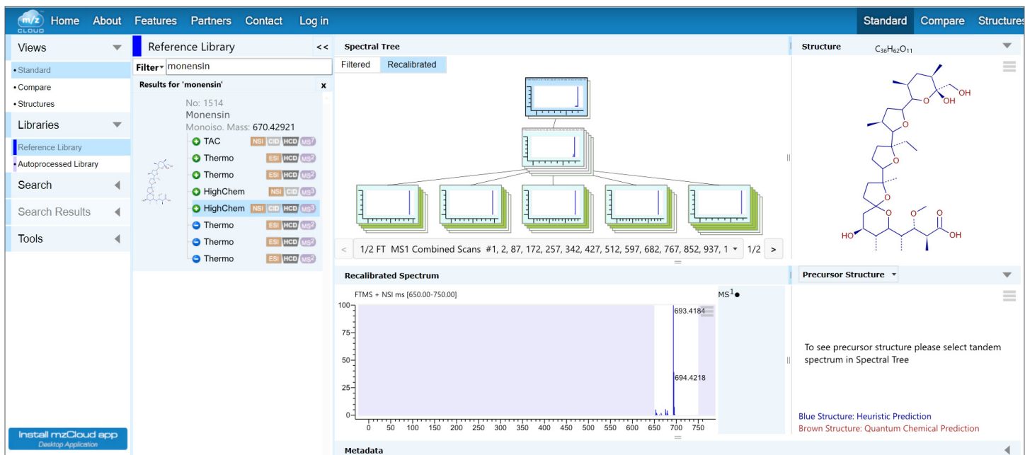
Figure 1. Screen capture from mzCloud showing the Monensin entry. The interactive entry enables multiple spectral views based on the instance for ionization polarity and MS n stage performed and form of dissociation used to generate the resulting ion tree.
