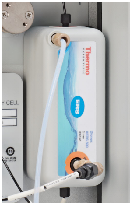
Figure 22. ERS 500 Suppressor installed
