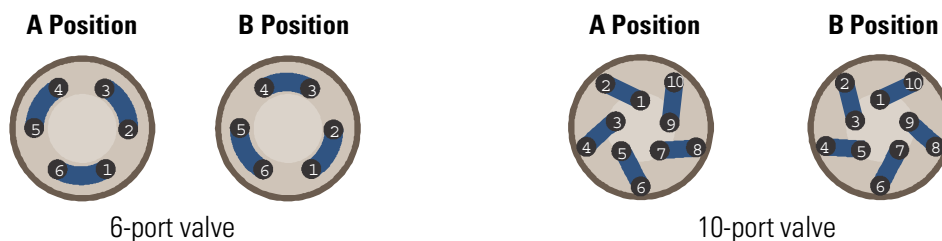
Figure 14. 6-port and 10-port high-pressure valve flow schematics
