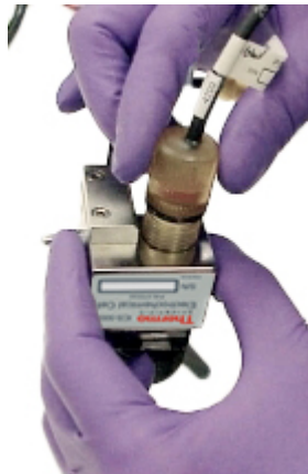
Figure 100. Installation of the pH-Ag/AgCl reference electrode in the reference electrode well
