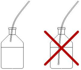
Figure 18: Free end of waste line in waste container
