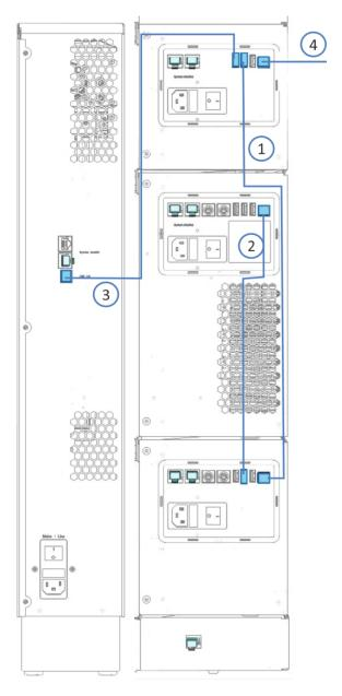
Figure 24: USB cable connections (example)
