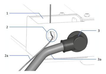
Figure 13: Funnel and waste outlets on the system base
