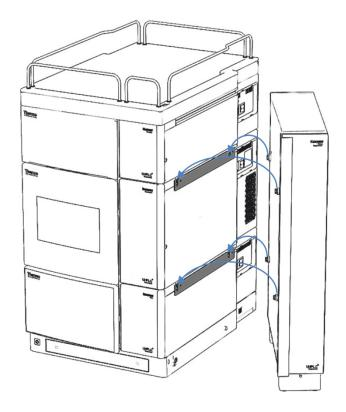
Figure 21: Attaching the column compartment to the system stack
