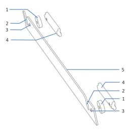
Figure 19: Mounting bar
