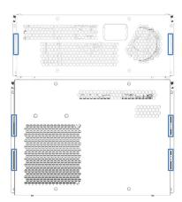
Figure 27: Cable clips in the autosampler and detector
