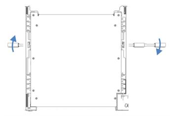
Figure 11: Locking the system base (system base top view)
