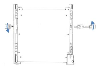
Figure 10: Unlocking the system base
