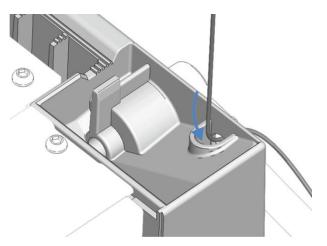
Figure 16: Routing the waste line through the outlet
