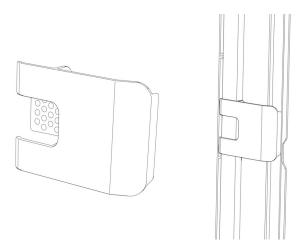
Figure 30: Tubing bracket (left), tubing bracket installed (right)
