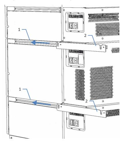
4. Tighten the screws on the mounting bars.
