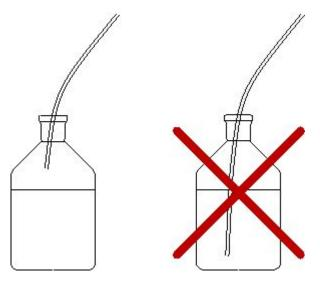
Figure 15: Free end of waste line in waste container
