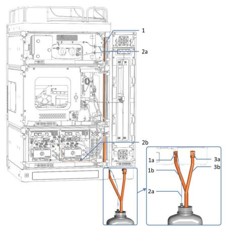
Figure 12: Overview of waste lines in the system (example)
