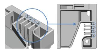
Figure 29: Tubing chase with tubing guides (left: view from inside, right: view from top)
