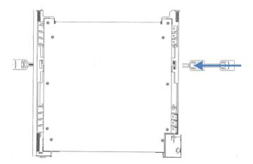
Figure 9: Inserting locking tools into the system base (system base top view)
