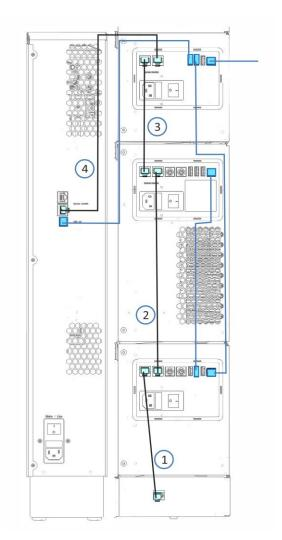
Figure 26: USB and system interlink cable connections (example)
