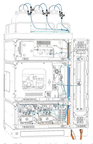
Figure 28: Flow connections in the Vanquish system (example)
