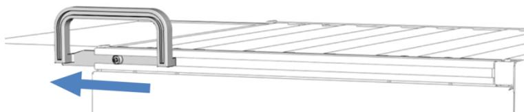
Figure 5: Sliding off the carrying handle from the left rail
