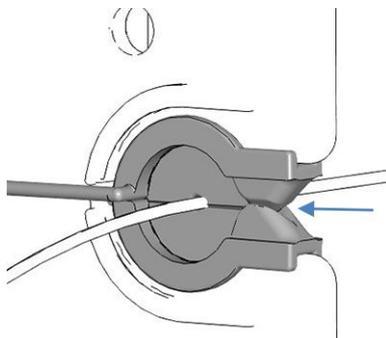
Figure 16: Capillary installed in the plug with slit
