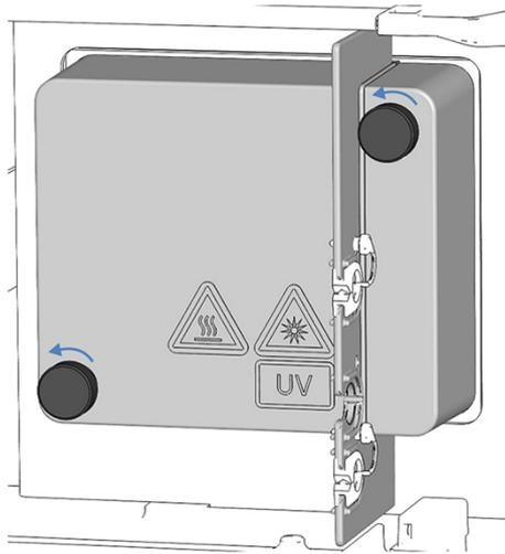
Figure 25: Screws on the lamp house cover
