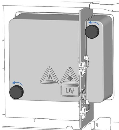
Figure 23: Screws on the lamp house cover
