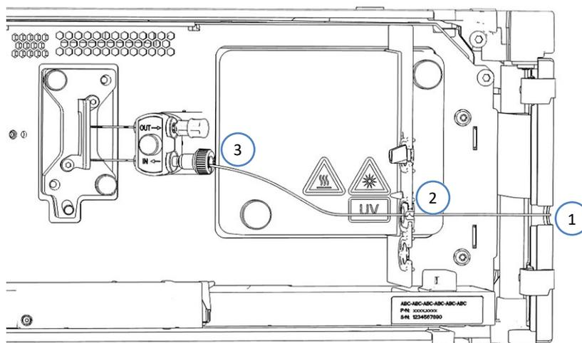
Figure 19: Connecting the inlet capillary from the column compartment (example)
