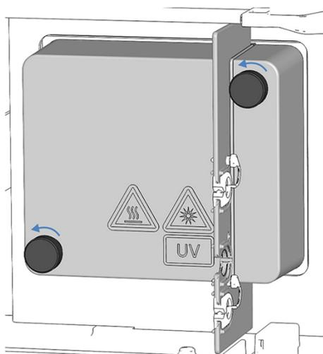
Figure 10: Screws on the lamp house cover
