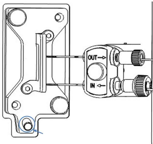
Figure 31: Flow cell drain outlet
