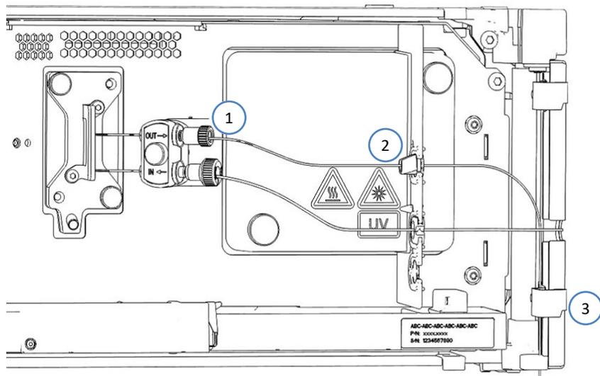
Figure 20: Connecting the detector waste line
