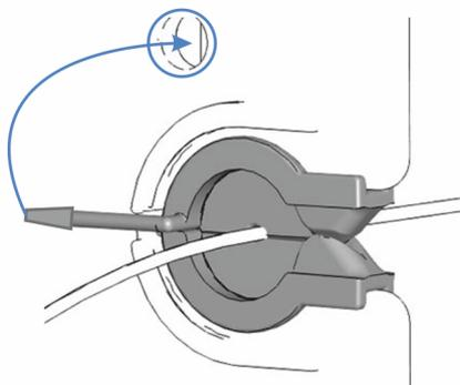
Figure 15: Securing the partition panel plug with slit
