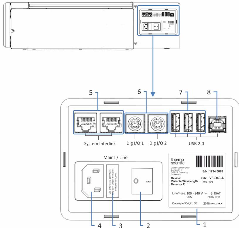
Figure 8: Electrical connectors on the right side of the detector
