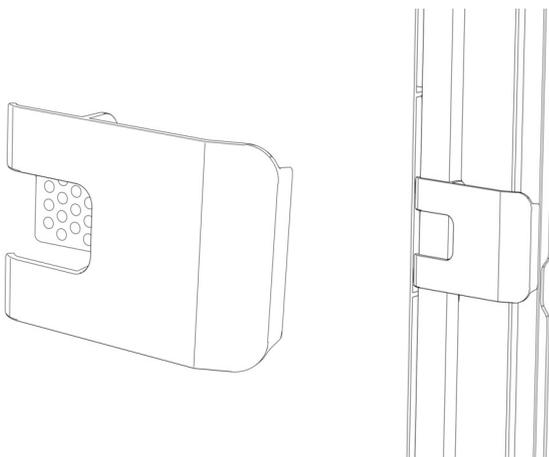
Figure 13: Tubing bracket (left), tubing bracket installed (right)
