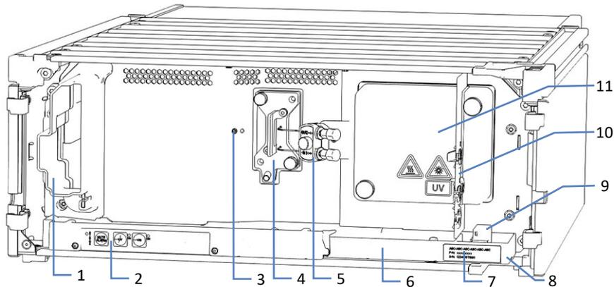
Figure 2: Interior components (here with flow cell with connection unit installed)
