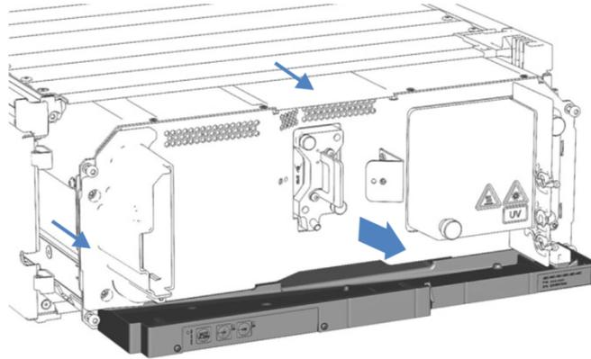
Figure 29: Pulling out the slide-in module (doors not shown)
