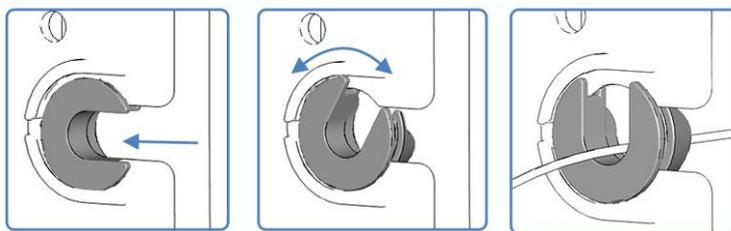
Figure 17: Using the rotating plug
