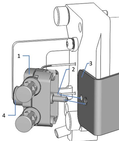
Figure 11: Installing a flow cell with connection unit
