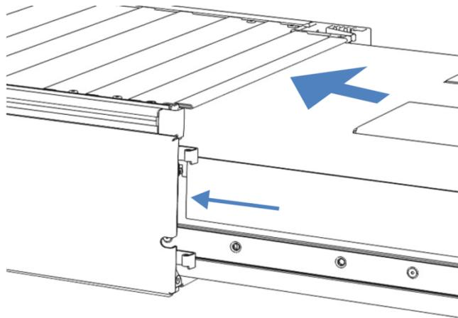
*Figure 30: Inserting the slide-in module*
