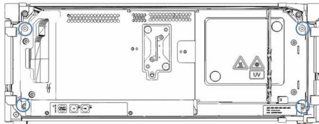
Figure 28: Captive screws on the slide-in module (doors not shown)
