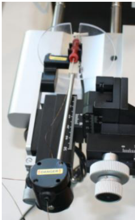
Figure 78. Column assembly mounted on DirectJunction
