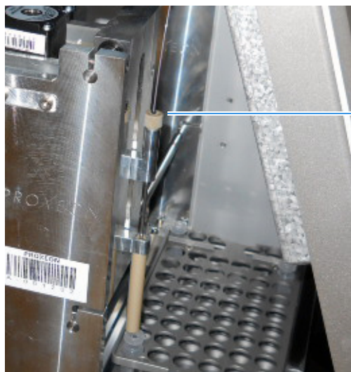
Figure 176. O-ring pushed slightly above the ASC needle holder
