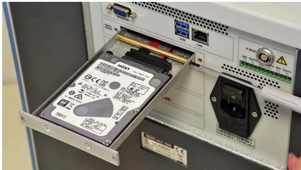
Figure 82. Removing the brass rod that holds the cable down
