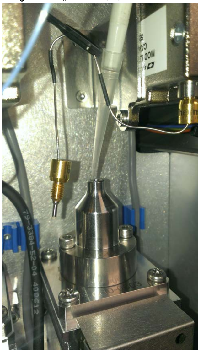
Figure 7. Adding solvent to the pump head
