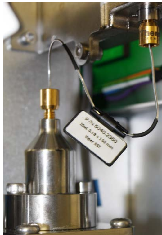
Figure 2. Stainless steel fitting removed from the pump head
