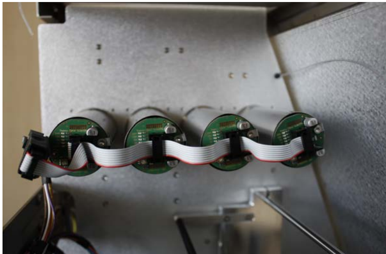
Figure 104. Cables connected to valves
