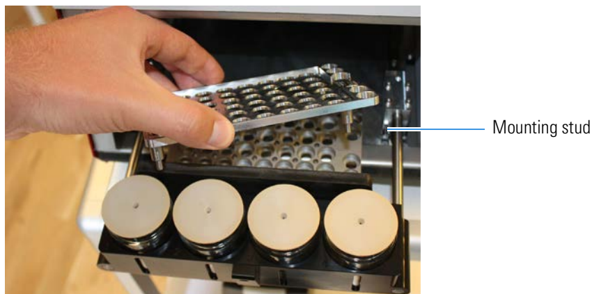
Figure 171. Removing the vial adapter plate before installing the MTP adapter plate.
