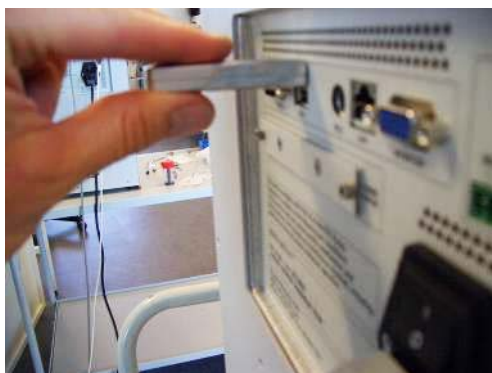
Figure 183. USB port location on the back panel of the EASY-nLC instrument
