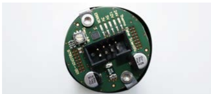
Figure 107. Schematic illustration of the valve address switch: Address shown is 3.
