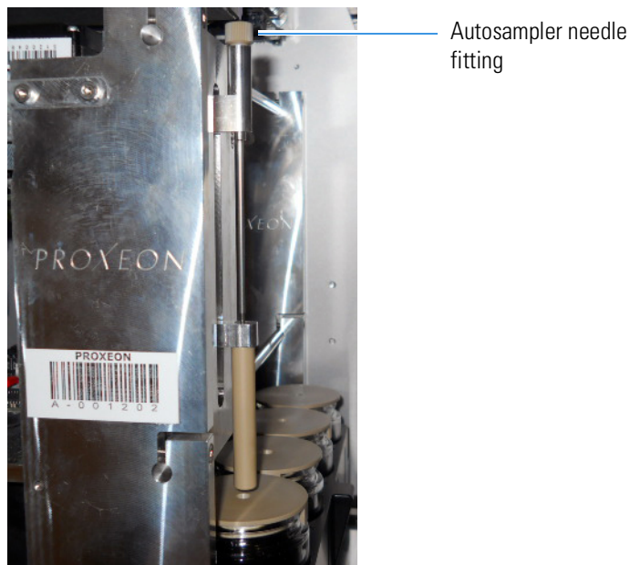
Figure 90. Needle connected to the needle holder
