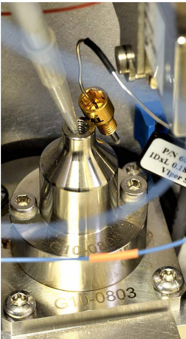
Figure 63. Adding solvent to the pump head
