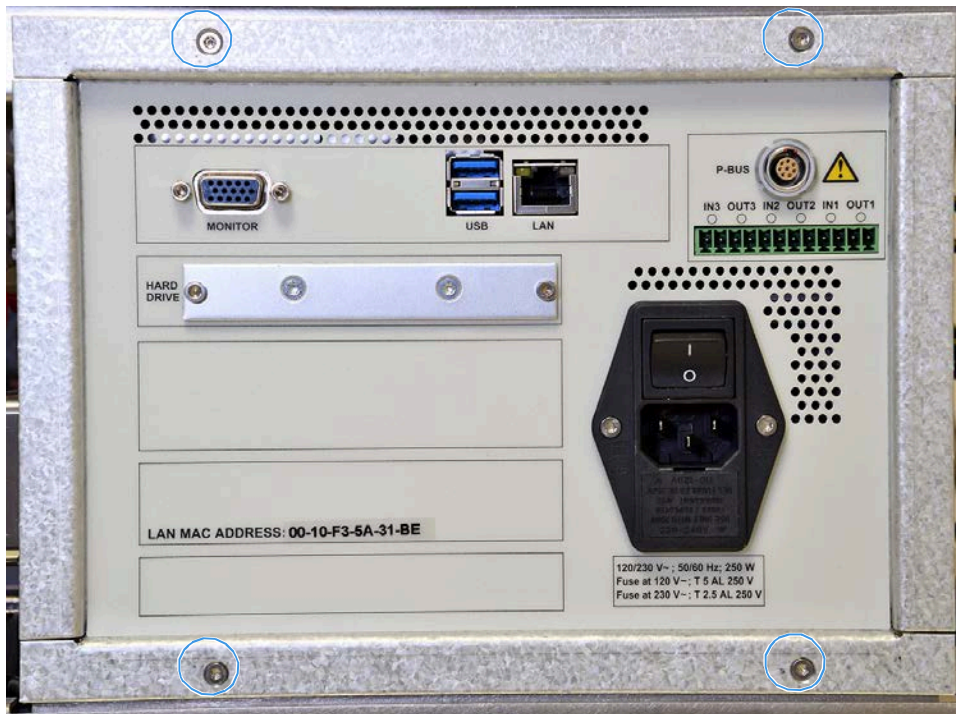
Figure 85. Screws to remove from the computer box
