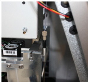
Figure 4. Autosampler needle connected to the z-axis needle holder
