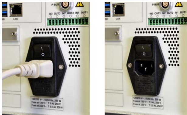
Figure 50. Power cable removed from the instrument's power receptacle
