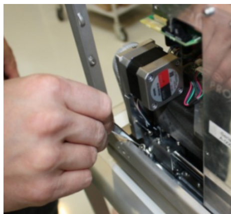
Figure 95. Removing the screw from the right side of the autosampler
