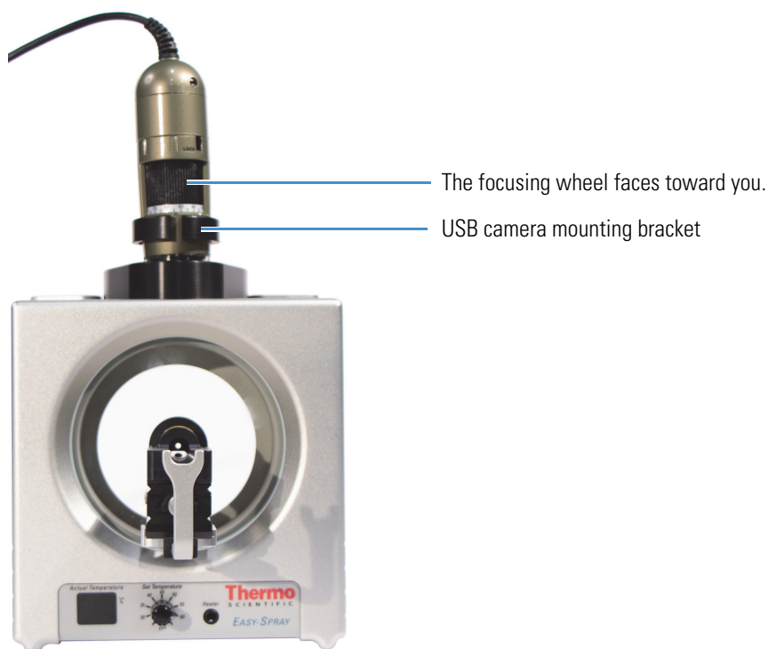
Figure 9. USB camera installed on the EASY-Spray ion source
