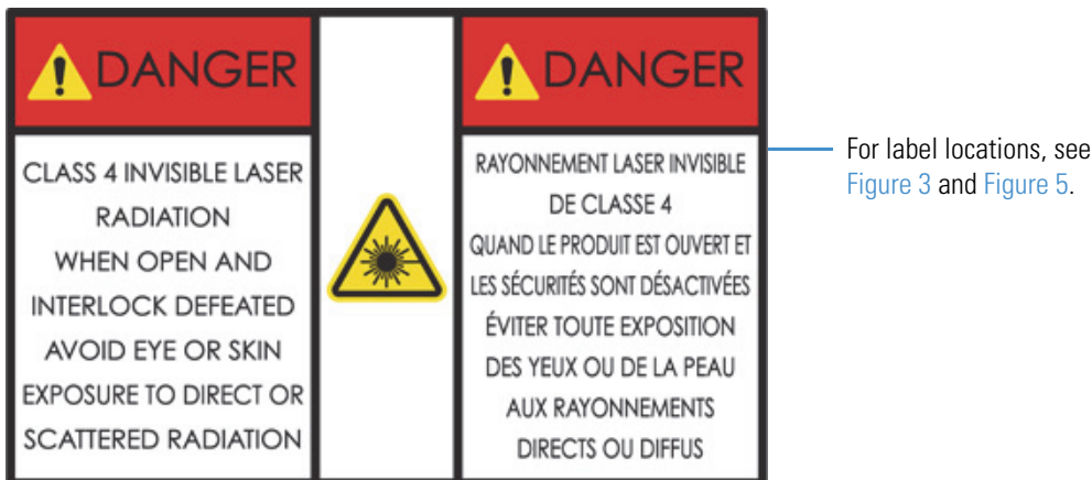
Figure 30. Laser head's Class 4 laser safety label
