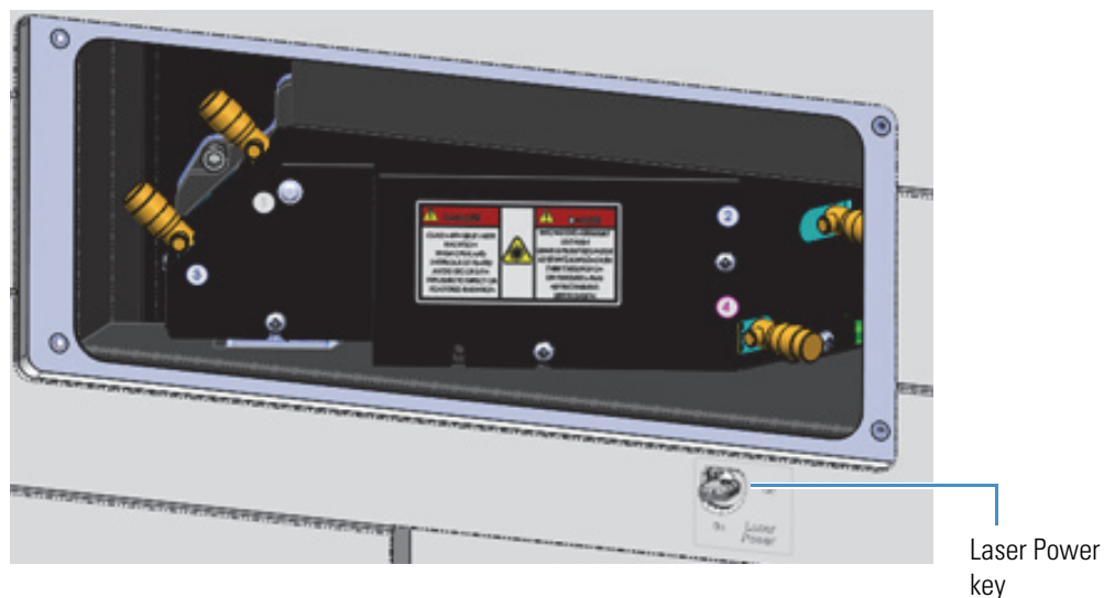
Figure 20. Laser module compartment with door removed
