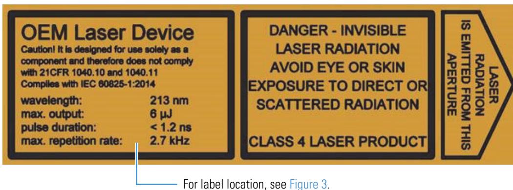
Figure 30. Laser head's Class 4 laser safety label
