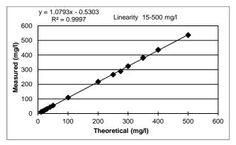
Linearity example is measured with Gallery analyzer. Arena analyzer shows similar performance.
