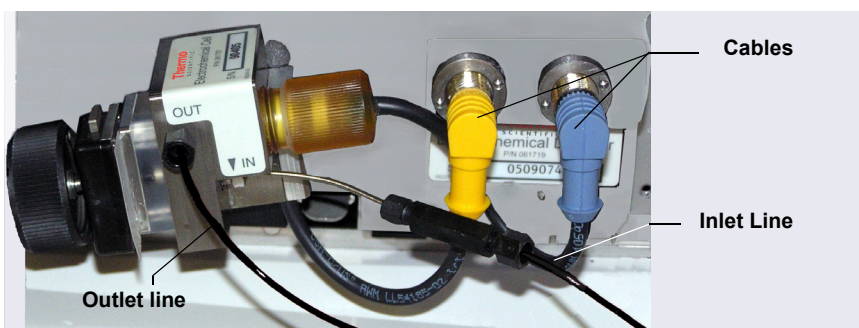
Figure 10-59. Disconnecting the ED Cell (Cell Configured for Analytical IC Shown)
