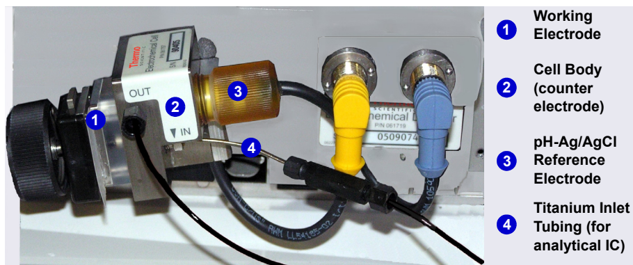
Figure 2-31. ED Cell with pH-Ag/AgCl Reference Electrode (Cell Configured for Analytical IC Shown)
