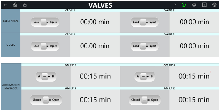
Figure 6-6. Valves Page for a System with Four Valves.
