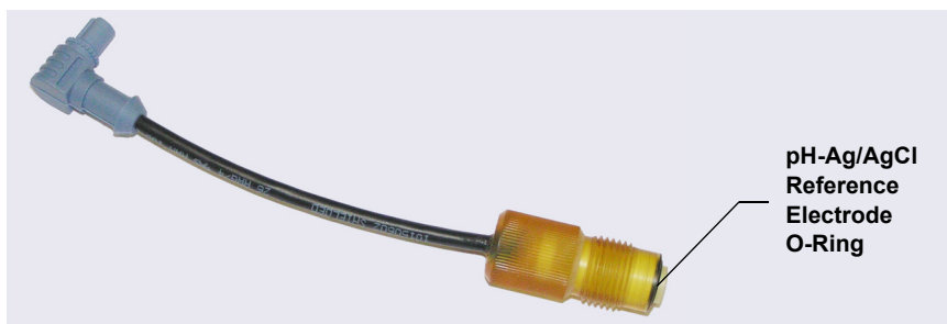
Figure 10-70. Removing the pH-Ag/AgCl Reference Electrode O-Ring
