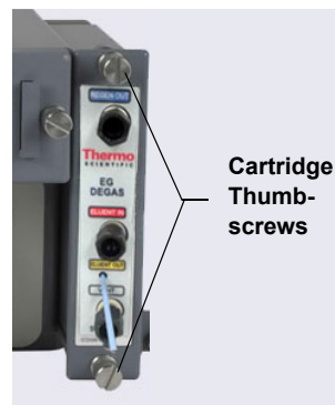
Figure 10-45. Capillary Cartridge Thumbscrews (EG Degas Cartridge Shown)
