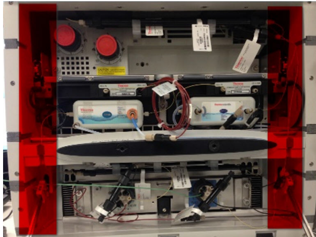
Tags should not be placed in the areas shown in red (the far left or far right side of the compartment)
