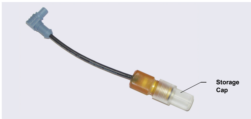
Figure 7-2. pH-Ag/AgCl Reference Electrode in Storage Cap
