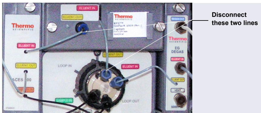
Figure 10-48. Disconnect Capillary Tray Eluent Lines (Conductivity System Plumbing Shown)
