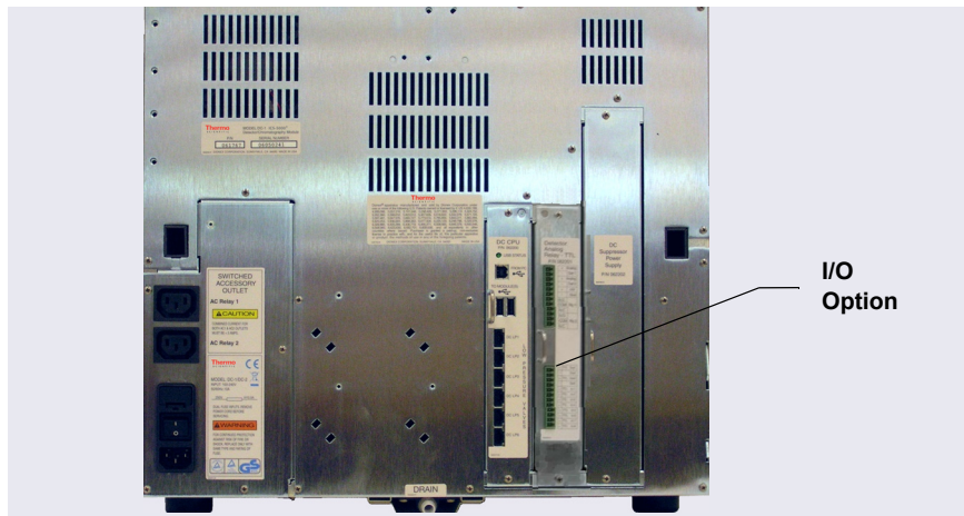
Figure 10-40. DC Rear Panel: I/O Option Installed
