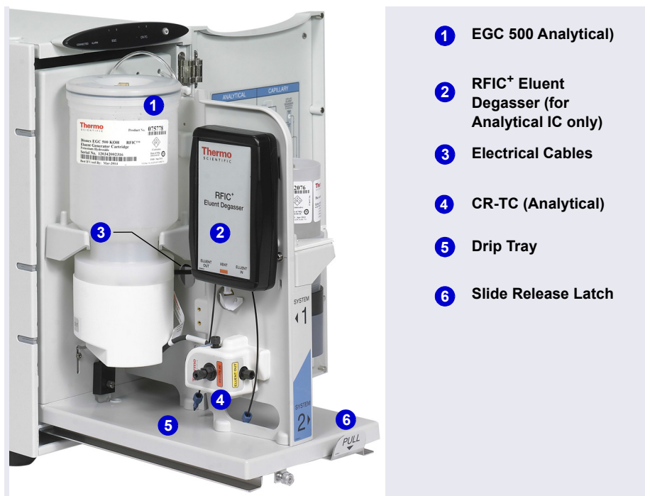
Figure 2-11. Example EG Interior Components for an Analytical (High-Pressure) IC System (System 1 Shown)
