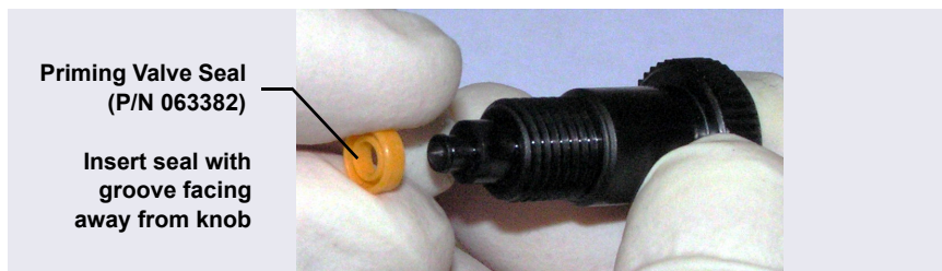
Figure 10-13. Replacing the Priming Valve Seal
