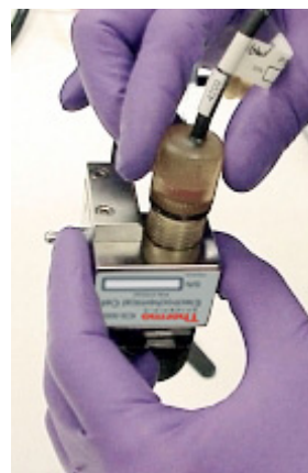
Figure 10-67. Installing the pH-Ag/AgCl Reference Electrode In the Reference Electrode Well
