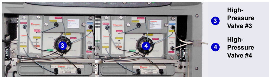
Figure 9-6. High-Pressure Valves #3 and #4 (in IC Cubes)
