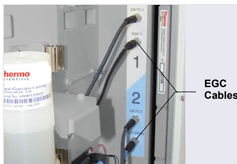
Figure 10-15. Dionex EGC Cables
