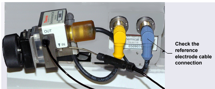
Figure 9-8. ED Cell Electrical Connections
