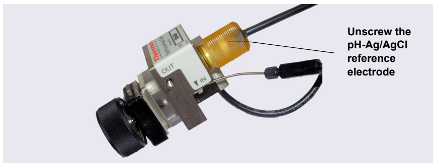
Figure 10-69. Removing the pH-Ag/AgCl Reference Electrode (Cell Configured for Analytical IC Shown)
