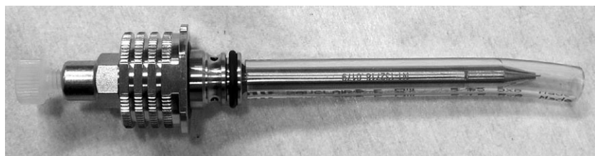
Figure 34: Nebulizer with protective tubing and plug on the flow inlet
