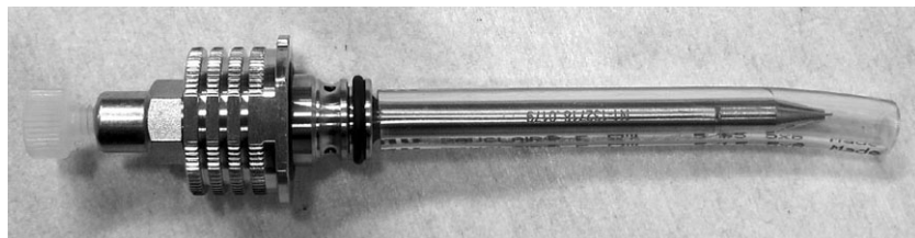
Figure 11: Nebulizer with protective tubing and plug on the flow inlet
