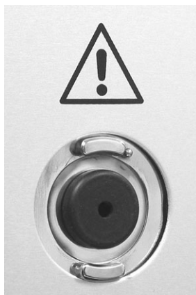
Figure 12: Dust seal plug installed in the nebulizer opening
