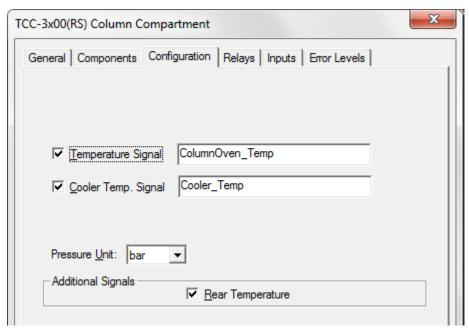
Fig. 12: Configuration page (here TCC-3000RS)
