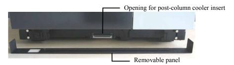
Fig. 22: Removable panel for post-column cooler
