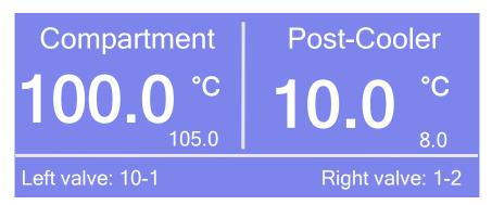
Fig. 42: Alternative status screen (here TCC-3000RS with two 2-position, 10-port switching valves)
