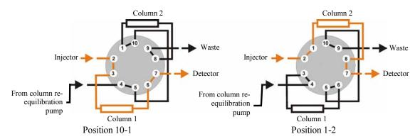
Fig. 5: Example for column switching with a 2-position, 10-port column switching valve
