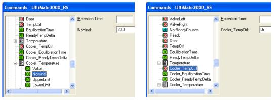
Fig. 40: Turning on post-column thermostatting
