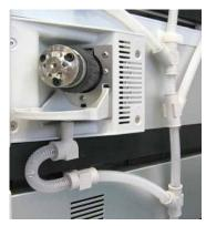
Fig. 16: Drip tray with drain tubing connected to the left valve and to the right valve
