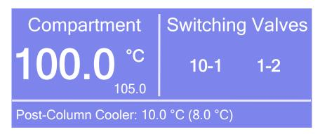
Fig. 31: Status screen (here TCC-3000RS with two 2-position, 10-port switching valves)
