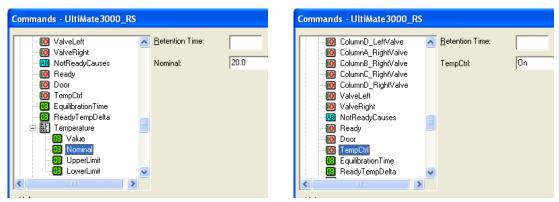
Fig. 39: Turning on column thermostatting
