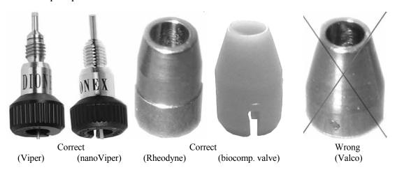
Fig. 44: Viper fitting connections and other valve ferrules (examples)
