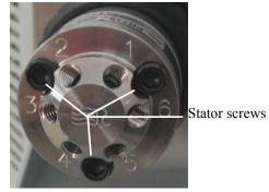
Fig. 51: Stator screws
