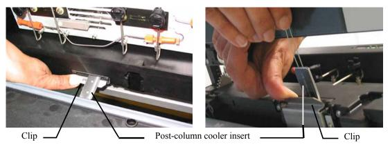
Fig. 23: Inserting the cooler insert (left: view from the top, right: bottom view)
