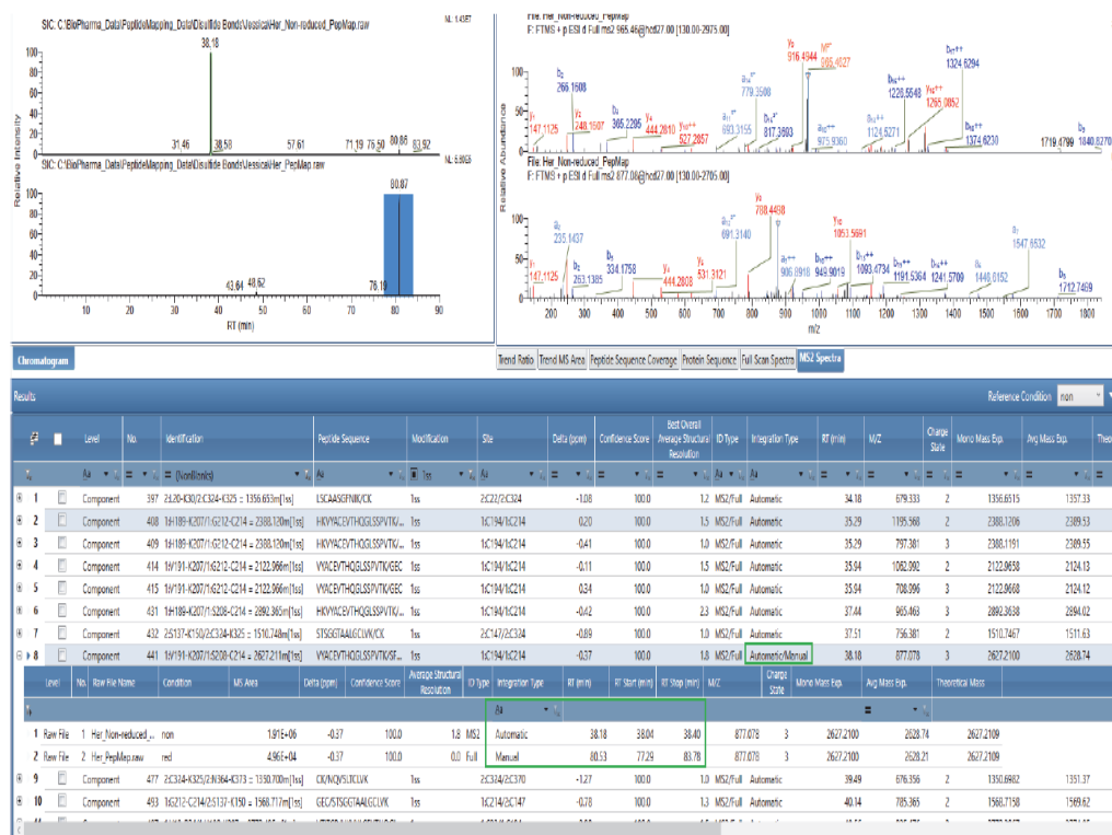
Figure 135 Manually integrated peak
