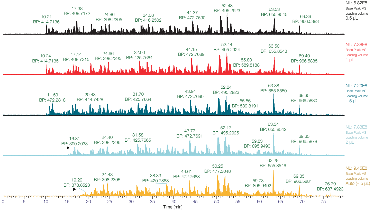
Figure 24. Base peak chromatograms obtained for the separation of 200 ng HeLa tryptic digest (1 \mu\text{L} injected) using different loading volumes. 50 cm \mu\text{PAC} Neo column, 67 min gradient. The loss of hydrophilic peptides at lower retention times is indicated by the arrows.
