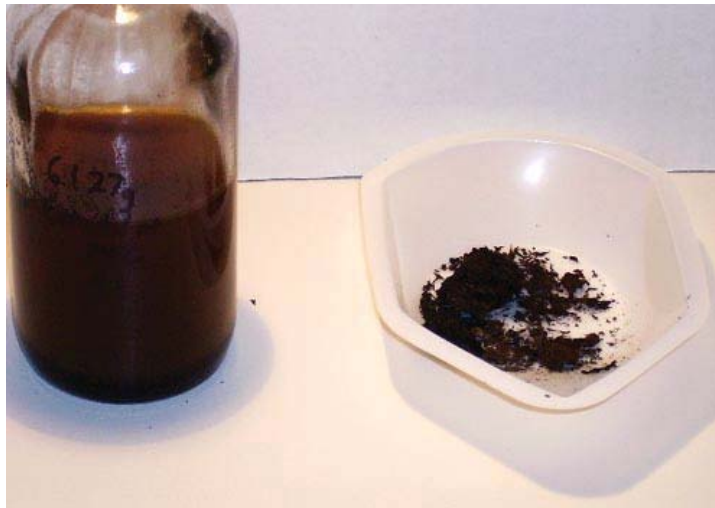
FIGURE 4. Dionex ASE 350 system extracts at 190°C with 0.1 M H 2 SO 4 .
