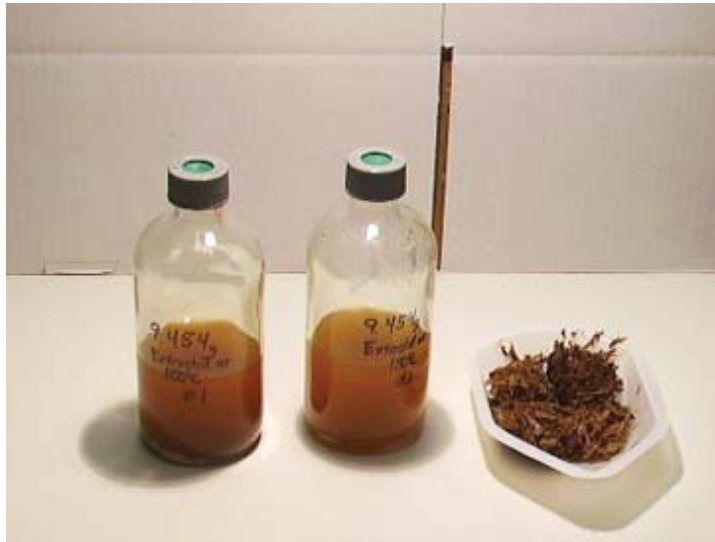
FIGURE 3. Dionex ASE 350 system extracts at 150°C with 0.1 M H 2 SO 4 .
