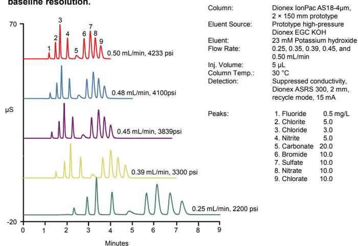
**FIGURE 7. Determination of inorganic anions in water samples using a prototype Dionex IonPac AS18-4 $\mu$ m 2  $\times$  150 mm column. Five anions in municipal or mineral water samples were eluted within 4 min on the 4  $\mu$ m particle size column, emphasizing the fast sample runs possible with this column.**
