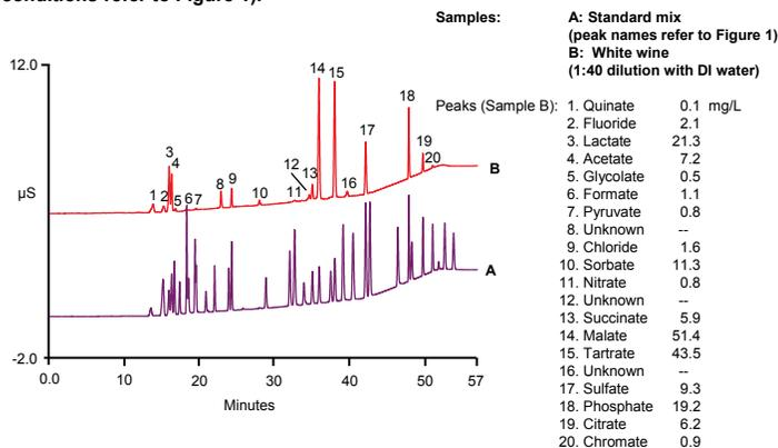
**Prototype 2 mm i.d. Dionex IonPac AS18-4 $\mu$ m Analytical Column**
