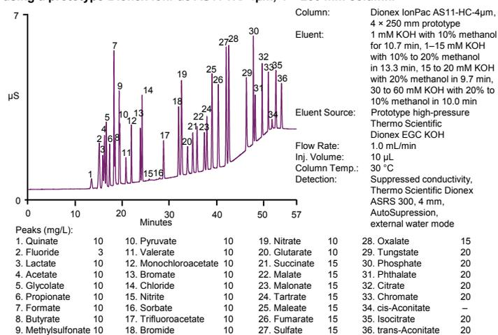
**FIGURE 2. The Dionex IonPac AS11-HC smaller-particle-size (4  $\mu$ m) analytical column provides improved resolution over the AS11-HC bigger-particle-size (9  $\mu$ m) analytical column, including improved separation for monovalent carboxylic acids, such as lactate and acetate, and better baseline resolution for bromate/chloride, formate/butyrate, methylsulfonate/pyruvate, and phosphate/phthalate (see Table 1).**
