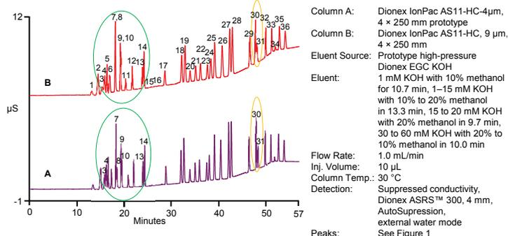
**TABLE 1. Comparison of resolution obtained on both columns with different particle size**
