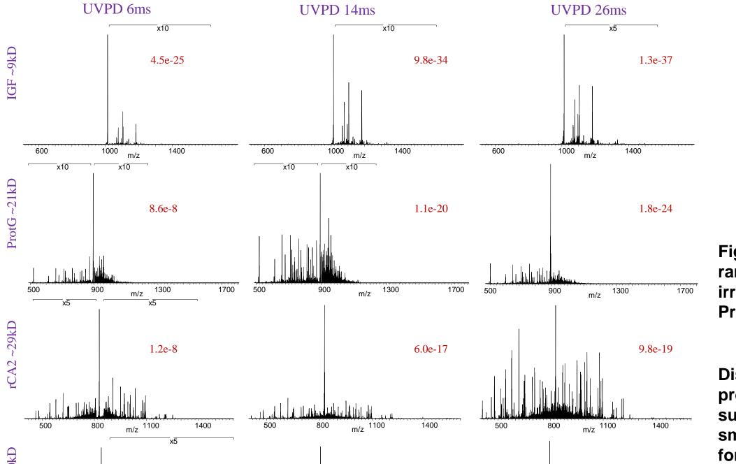
Figure 5: UVPD analysis of 4 different proteins ranging in MW from 9kD to 50kD, at 3 different irradiation times. Inset numbers in red are ProSightPC P-scores.
