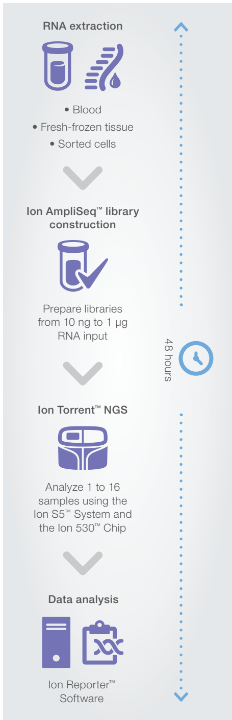
Figure 1. Workflow overview. Manual library construction is followed by automated template preparation using the Ion Chef™ System. Sequencing is performed on the Ion S5 System with data analysis using Ion Reporter Software.
