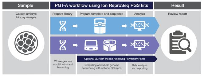
A premium PGT-A workflow on the the Genexus sequencer (blue) or Ion GeneStudio S5 systems (purple) with Ion ReproSeq PGS kits and the Ion AmpliSeq Polyploidy Panel. This workflow easily combines aneuploidy analysis with SNP-based QCs by integrating sequencing and analysis in a single platform.
