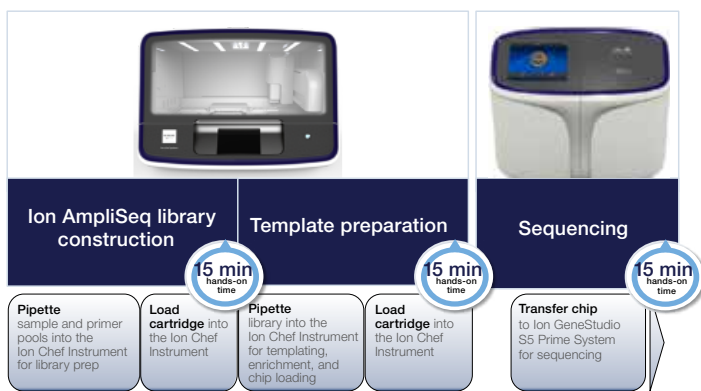
Figure 2. Streamlined workflow for gene expression analysis. Fully automated workflow from cDNA to gene expression data requires only 45 minutes of hands-on time using the Ion Chef System and Ion GeneStudio S5 Prime System.
