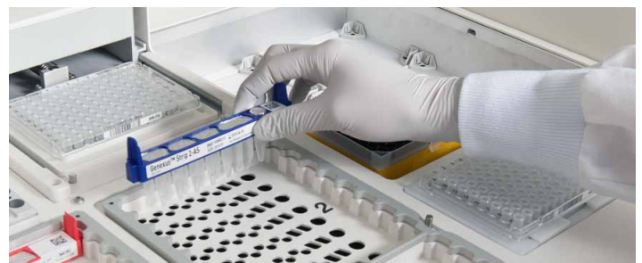
Figure 5. Loading reagents into the Genexus system.
