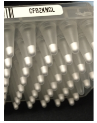
Figure 8. Lyophilized Reactions in a 96-well plate
