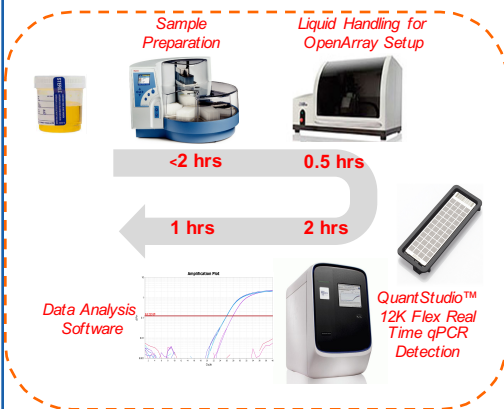
Figure 1: Complete Workflow Solution: Sample to answer in less than 5.5 hours. Each OpenArray™ plate consists of 48 subarrays each containing 56 TaqMan™ assays spotted according to customer's specifications. Up to 4 OpenArray™ plates can be included in a single QuantStudio™ 12K Flex run allowing for a throughput of 192 samples.
