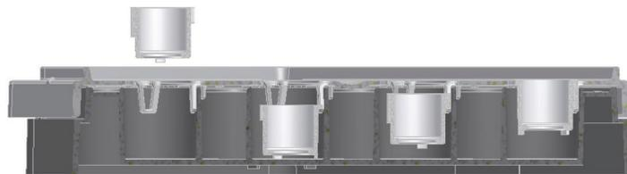
Figure 4. Cross-sectional view of the Nunc Carrier Plate with 3 hanging positions for the Nunc Cell Culture Inserts.
