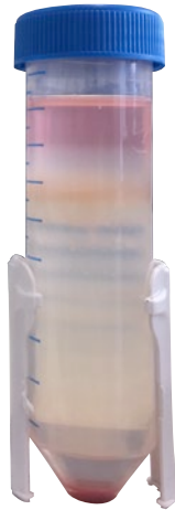
Figure 3. Density gradient centrifugation. Cytotrophoblast cells are located in the cell layer corresponding to 1.048 g/mL–1.060 g/mL density.
