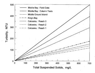
If it is desirable to match the online SS sensor readings to the laboratory TSS results, there must be a sample-specific calibration of the SS sensor. This can be done by generating a correlation or by a calibration update, according to user preference.
