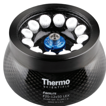
Figure 2. The Thermo Scientific Fiberlite F20-12x50 LEX rotor.
