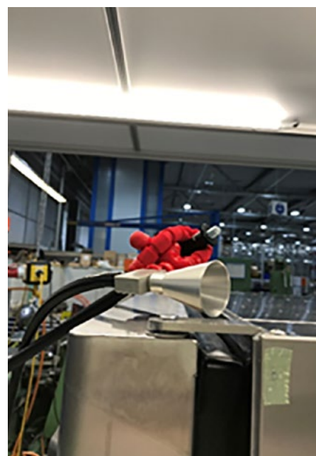
Figure 6. Heracell Vios 160i CR at the highest emission point MP 3, located on the upper right side, above the top door hinge.
