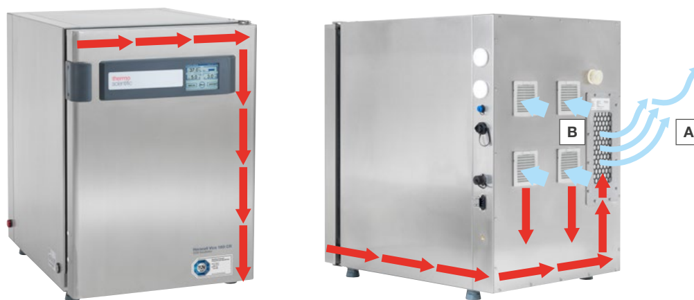
Figure 2. Overview of the process used to test CO 2 incubator suitability for use in a cleanroom, in accordance with ISO 14644-14: 2016. A measuring point with the highest particle emissions detected was located at the upper right side, above the top door hinge. This point was used for the final ISO class compatibility determination.
