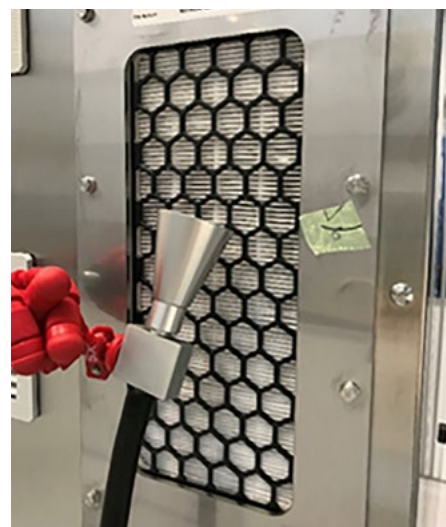
Figure 5. MP 6, on the back of Heracell Vios 160i CR, close to the HEPA filter.
