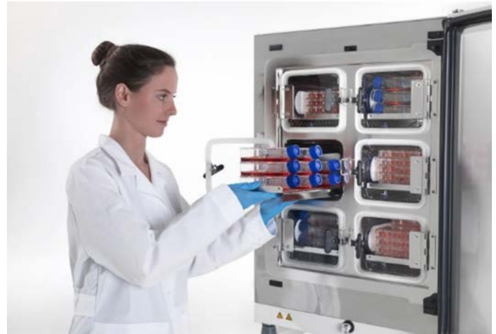
Figure 1: Cell Locker System Segregates Cultures or Projects. Cell Locker System consists of six individual protected chambers inside a Heracell VIOS 160i or a Forma i160 Steri-Cycle CO 2 incubator. 0.2 µm filter membranes permit air exchange but protect from cross-contamination and maintain ideal conditions.
