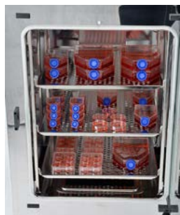
Figure 3: A typical laboratory has conditions far different than in a typical CO 2 Incubator. During a door opening, conditions in any incubator drop close to those in the surrounding room. In this example, the CO 2 incubator is set to 37°C, 5% CO 2 , 1% oxygen, 93% humidity but these parameters drop swiftly during a thirty second door opening. In a Cell Locker System, ideal conditions are maintained when a neighboring Cell Locker Chamber is opened to remove cultures.
