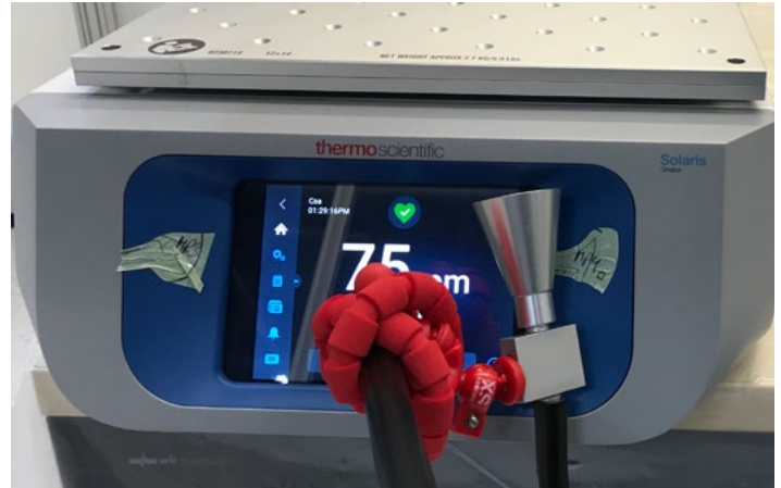
Figure 1: In accordance with the ISO 14644-1 and VDI 2083 standards, an orbital shaker should be tested for particle emission from all suspected particle hot spots, like edges, seals and openings. 3,4
