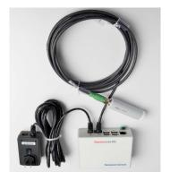
CO<sub>2</sub> Sensor Connected to DeviceLink Connect Mote
