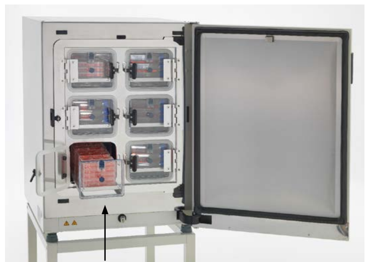
Figure 1: The Cell Locker System inside a Heracell VIOS CO 2 Incubator provides six segregated isolation chambers for critical cells or projects inside a single incubator. The inner transport door (black arrow) is optional and can be removed. The inner incubator door is segmented such that each Cell Locker Chamber has its own individual door, but the entire inner door can be opened, providing access for cleaning.
