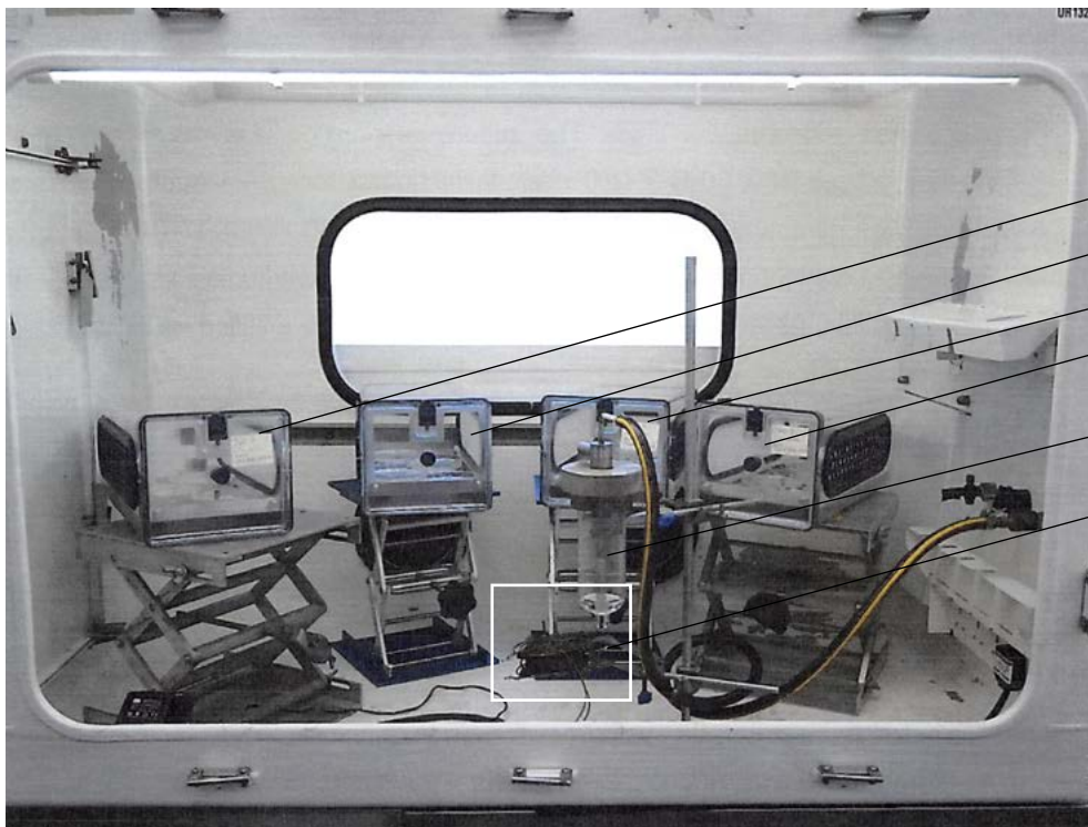
Figure 5: Four Cell Locker Chambers with the optional transport door, and three different door gaskets, were positioned inside an MSC III cabinet. A nebulizer sprays the bacterial suspension and a small circulating fan helps to disperse the bacteria. Each Cell Locker Chamber contains four opened TSA plates inside and one opened TSA plate on top.
