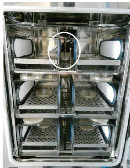
Figure 4A: Nebulizer placement in the Cell Locker System. The tubing was led through the access port in the upper left back wall of the incubator.
