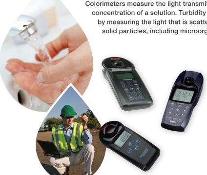
Colorimeters can be used to measure the amounts of disinfectants and their byproducts, and the concentration of various inorganic and organic chemicals. Turidimeters help to determine the number of microorganisms in the water, or to measure cloudiness caused by flooding and run-off.
