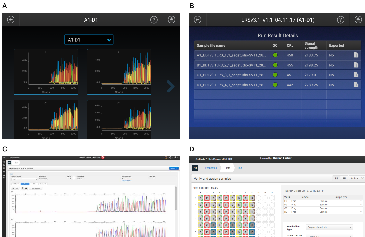
Figure 1. Real-time monitoring of runs on the SeqStudio Genetic Analyzer. (A) The SeqStudio instrument displays results for each capillary in real time. (B) Once an injection is finished, a number of quality checks are calculated and displayed. If an injection produces poor traces or poor QC values, those samples can be reinjected, with altered injection parameters, if desired. (C) Screenshot from an off-site computer monitoring shows the progress of a run. (D) Runs set up in PlateManager can be uploaded directly to the instrument. PlateManager allows investigators to assign sequencing and fragment analysis runs on the same plate, taking advantage of the universal polymer in the cartridge.
