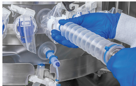
Figure 3. Bioreactor probe assembly.
