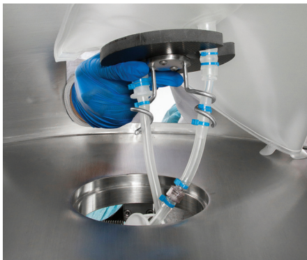
Figure 4. Sparge line support.
