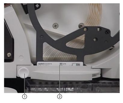
Figure 36 Array header latch and array housing
