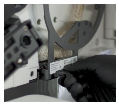
Figure 79 Slide the array header into the housing
