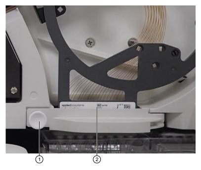
Figure 80 Array header latch and array housing
