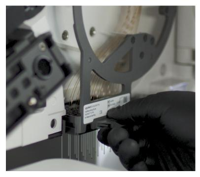
Figure 46 Tab on capillary array
