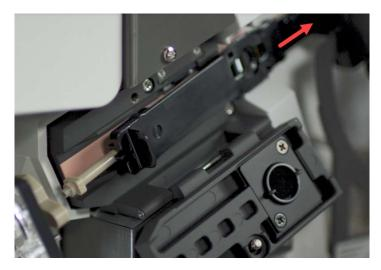
Figure 37 Slide the retractor tab to the right
