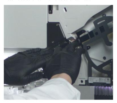
Figure 57 Press the detection cell into the detection cell heater
