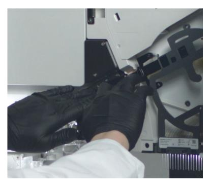
Figure 39 Press the detection cell into the detection cell heater
