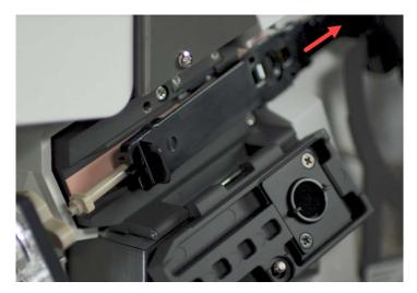
Figure 55 Slide the retractor tab to the right
