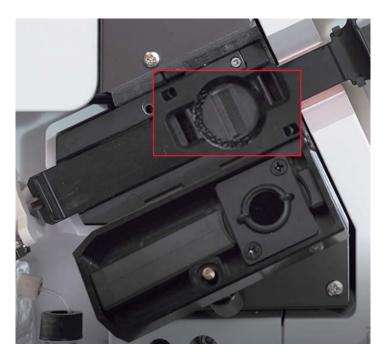
Figure 3 Detection cell heater with the door open and a capillary array installed. The detection cell in the capillary array is shown in the red box.
