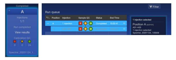
**Note:** If data for a capillary is borrowed, it is listed in the  $\diamond$  (caution) category. Example of Calibration QC with a borrowed capillary:
