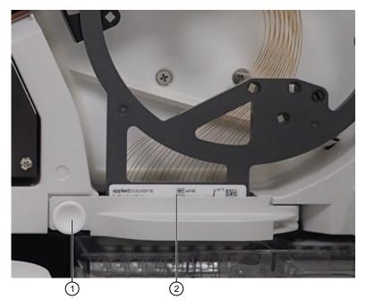
Figure 54 Array header latch and array housing
