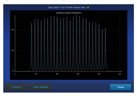
Figure 16 Example 24-capillary array spatial calibration profile
