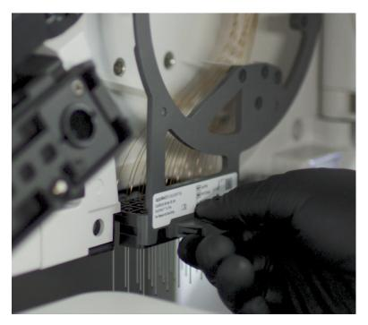
Figure 72 Tab on capillary array
