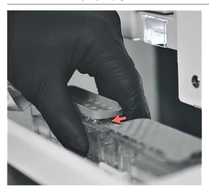
6. Wipe away condensation on the new CBC exterior with a lint-free tissue. Condensation can cause arcing and termination of the run.
