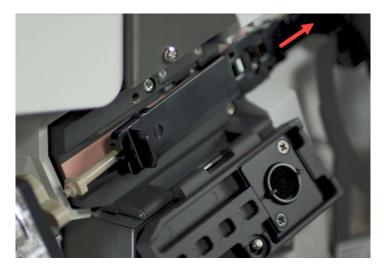
Figure 81 Slide the retractor tab to the right
