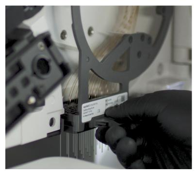
Figure 31 Tab on capillary array
