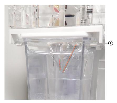
Figure 91 Examine anode channels for bubbles
