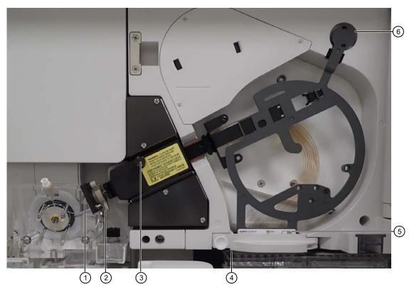
Figure 21 Capillary array with detection cell heater door closed
