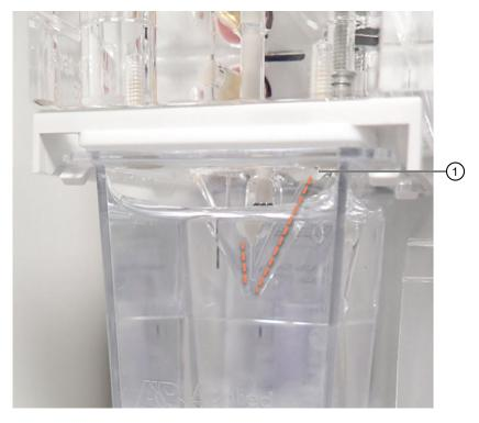
Figure 25 Examine anode channels for bubbles
