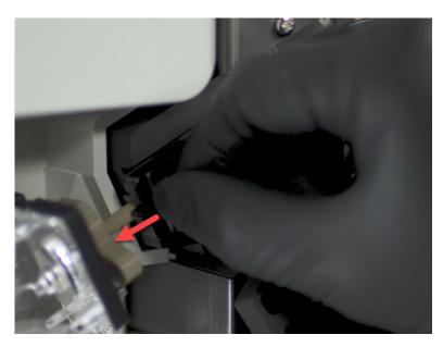
Figure 38 Insert the array tip into the array port
