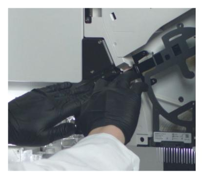
Figure 83 Press the detection cell into the detection cell heater
