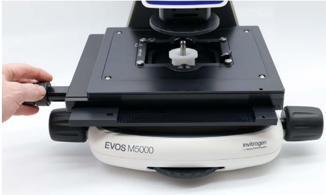
Figure 2 After removing the stage lock pin and moving the stage to access the shipping restraint.
