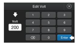
**4.** Set the operating mode parameter (Constant voltage) by entering the value in the Volt field, then select Enter.
