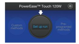
**1.** Turn on the power supply, then select **Set up run**.
