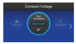
**8.** Completion of the run when the timer reaches 00:00∞ is indicated by an audible beeping alarm and a display of **Run Complete** ✓ in the center dial. Select **Home** to return to the home screen.
