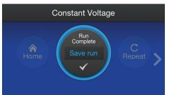
8. Completion of the run when the timer reaches 00:00∞ is indicated by an audible beeping alarm and a display of Run Complete ✓ in the center dial. Select Home to return to the home screen.
