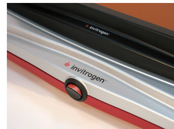
Figure 3. On / Off switch: Red mark is seen when on.
