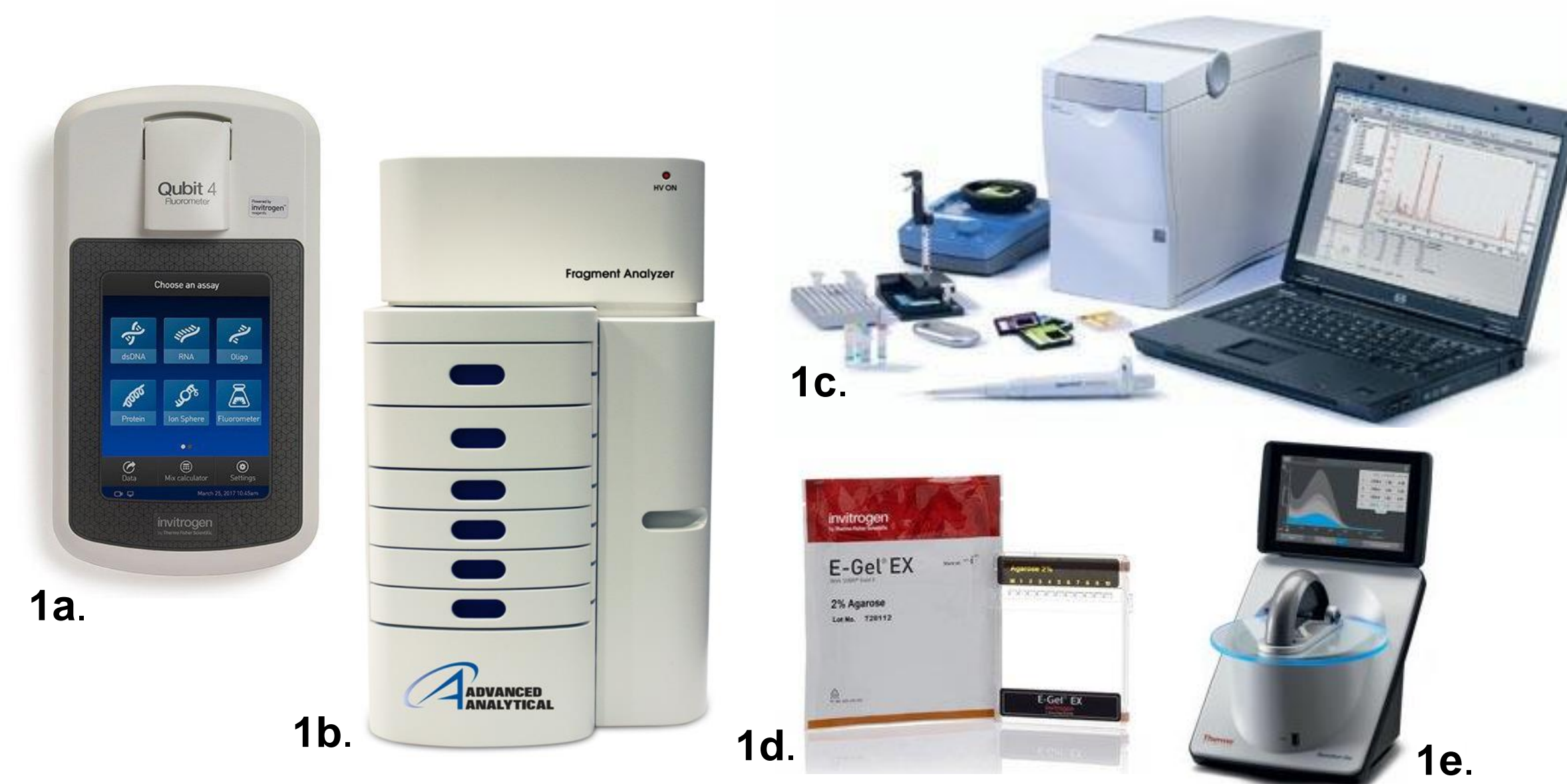
Figure 1: Methods for assessing RNA quality and quantitation 1a. Qubit 4: fluorescence signals from nucleic acid dyes. 1b. Fragment Analyzer: RQN score determined by capillary electrophoresis. 1c. Bioanalyzer: RIN score determined by capillary electrophoresis. 1d. E-Gel EX: gel-based separation and imaging methods. 1e. NanoDrop UV/vis absorbance
