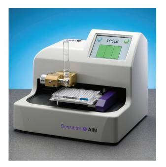
There have been no studies on aerosol generation using the Sensititre AIM<sup>™</sup> System or a multi-channel pipette. Therefore, a series of experiments were conducted to verify that the recommended inoculation methods for Sensititre products are safe when microbiologists follow standard laboratory procedures associated with BSL3-rated isolates.
