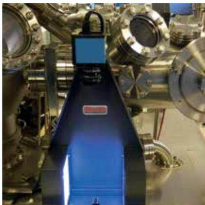
**Figure 1: The Platter Camera option, shown beside the sample loading door on the ESCALAB**
