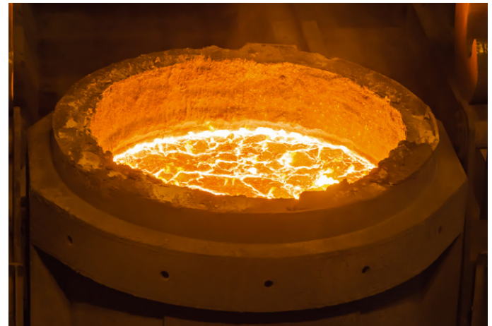
Figure 10. Refractory bricks line this ladle of molten steel at temperatures higher than 1,550°C while being corroded by slag.
