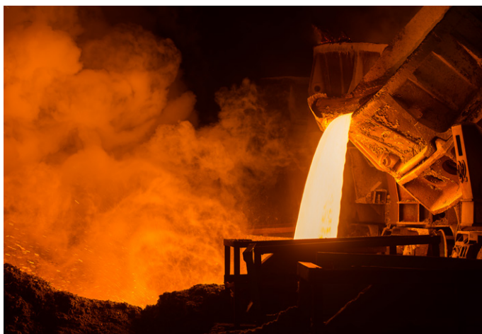
Figure 1. Refractories are used to contain the molten steel.
