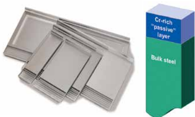
Figure 1: Passivated stainless steel samples and schematic of layer composition
