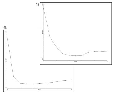
Figures 4a and 4b: Predicted Error Sum of Squares, or PRESS, plots for glutamine (4a) and glucose (4b).
