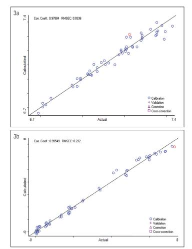
Figures 3a and 3b: Calibration curves for pH (3a) and glucose (3b).
